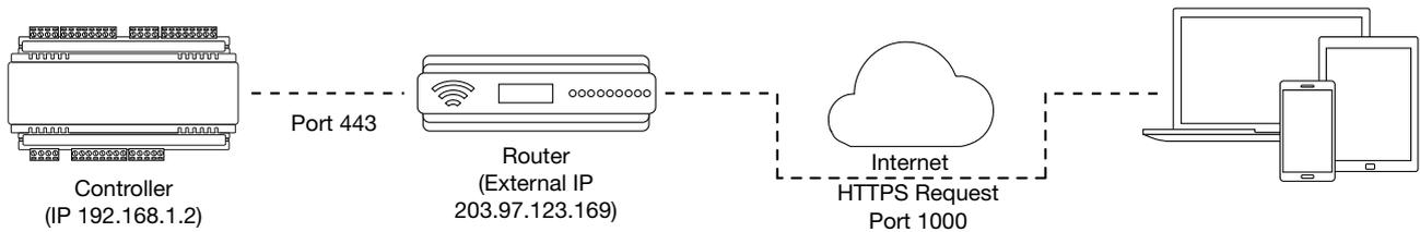
In this case, any traffic directed to **external port 1000** will be forwarded to the controller's HTTPS port. The controller's web interface can be accessed simply by appending the external port number onto the end of the URL: e.g. `https://203.97.123.169:1000`.
