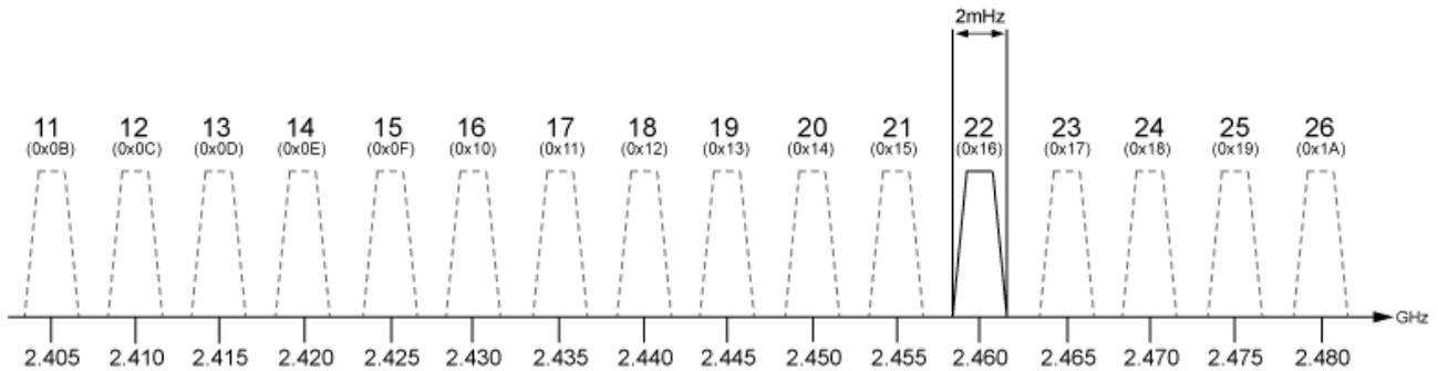
As an example, we can look at how Wi-Fi can affect the operation of SALLIS when it is operating on the same 2.4GHz band. Wi-Fi generally operates on a standard of the IEEE 802.11 communication protocol divided into 14 channels, each occupying 22MHz of bandwidth from 2412MHz to 2484MHz.
